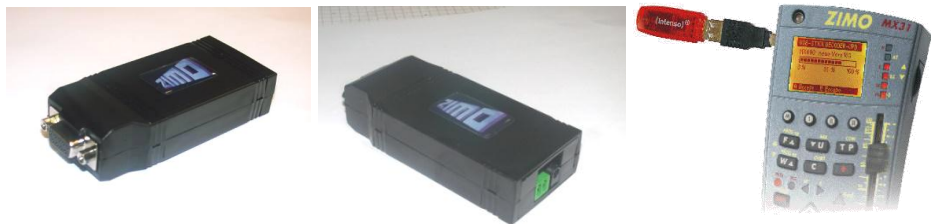
MXDECUP MX31ZL with USB-Stick RS-232 – DSUB-9-Plug Connector for update track control LED's behind socket Socket for power supply
